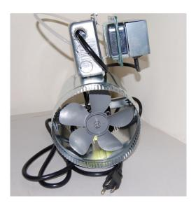
1. To install separate a joint in a branch duct. Cut off a length of duct 1 inch shorter than the duct fan being installed leaving 2 female ends to accept the duct fan. Both ends of Acme Miami duct fans are crimped. Seal both joints with Duct
